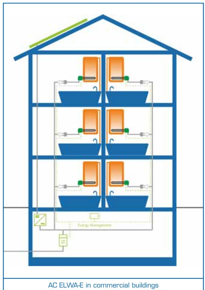
Decentralized hot water storage and production avoids distribution ("ring main") losses and fulfills hygienic standards.
